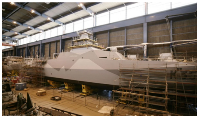
The Second Visby -class corvette Karlstad under construction (Photo credit: defencetalk.com)
