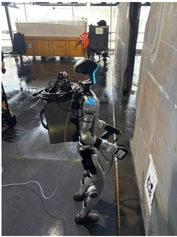
Fincantieri's Humanoid Welding Robot (Photo credit: Center for Maritime Strategy).
